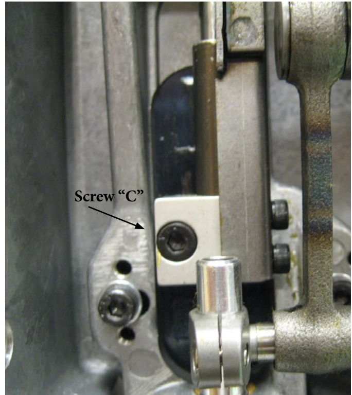
Figure 7 Inside view of Screw "C" (cover to be only removed by authorized Handi Quilter retailer).
