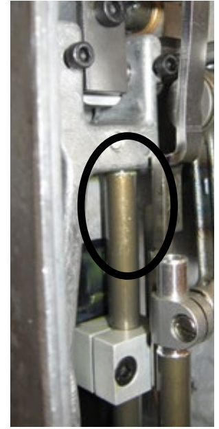
Figure 2 Raised position of the presser bar; spring-loaded plunger is compressed.
