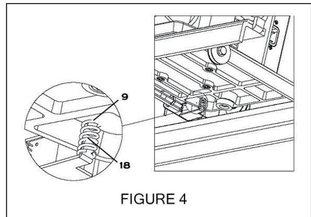
5. **To replace the wheel with the encoder assembly from the carriage do the following** (front encoder): remove the nut, washer, spring, encoder bracket, washer, bolt and wheel from the front encoder. Replace the encoder in reverse order or follow the directions as described below in 6 and 7.
