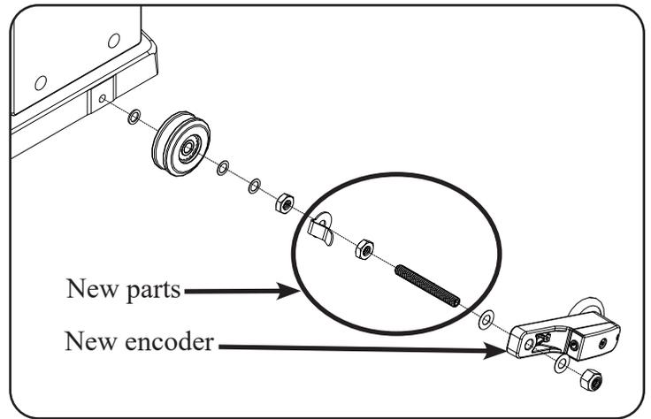
⚠ **IMPORTANT:** The encoder wheel must turn in order for stitch regulation to work properly. The magnetic encoder spring latch is used to hold the encoder up out of the way when the machine is removed from the carriage.
