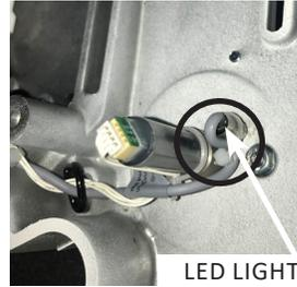
Notice the sensor cable is wire tied to the side of the sensor. This provides a little resistance when trying to move the sensor out.
