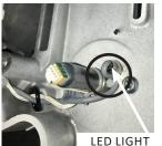
Notice the sensor cable is wire tied to the side of the sensor. This provides a little resistance when trying to move the sensor out.
