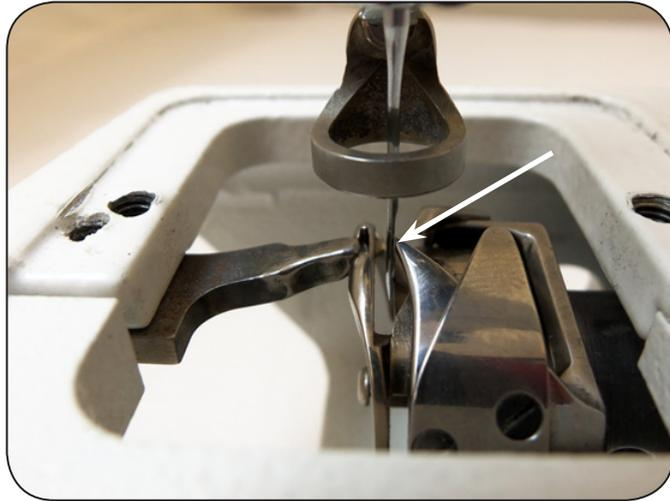
11. When the hook point reaches the far edge of the needle, the hook point should look like this relative to the needle eye. *This is the needle bar height.*
