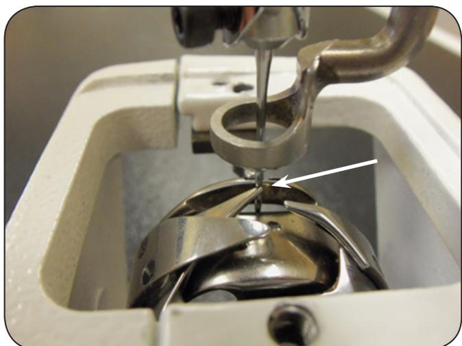
10. The hook point should be lightly brushing or touching the needle inside the scarf. *This is the needle distance.*
