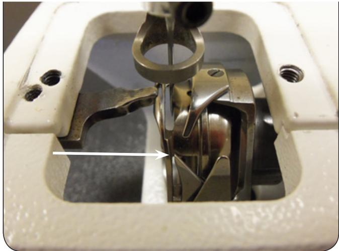
9. Slightly turn the handwheel in the direction of motion to raise the needle bar 2.2 mm. The hook point should reach the far edge of the needle. *This shows the loop lift.*
