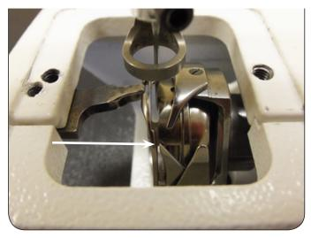
9. Slightly turn the handwheel in the direction of motion to raise the needle bar 2.2 mm. The hook point should reach the far edge of the needle. This shows the loop lift.
